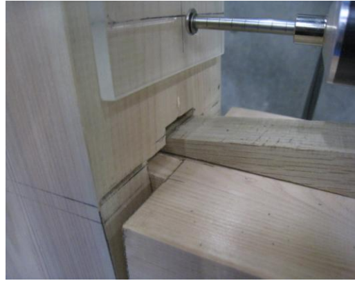
鼻-B-30hh(J-4-①hh2)柱-梁ずれ(1/8. 8rad)
