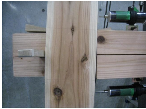
鼻-B-30ss(J-4-①ss5)ほぞせん断破壊(1/8. 8rad)
